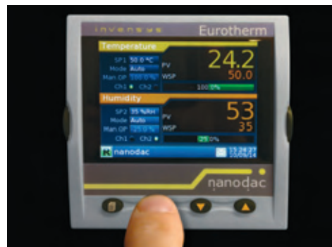
Push-buttons enable scrolling between configured views
